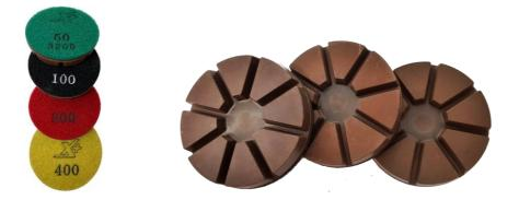
Grinding wet? AQUA ZERO pads from WORX+ have been designed to deliver more meters in the wet. Long life resin pads, rubber and Velcro backed to increase flexibility and smooth operation, with a highly consistent scratch pattern, are the choice for floor honing and polishing and wet cutting power-trowelled/burnished concrete where zero aggregate exposure is required before densification.
